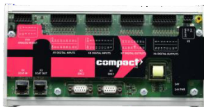
Compact I/O (Guide rail installation)
